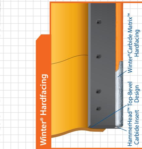
Three powder coated carbide insert blade segments with Winter® CarbideMatrix™ hardface reduces washout from end to end.
